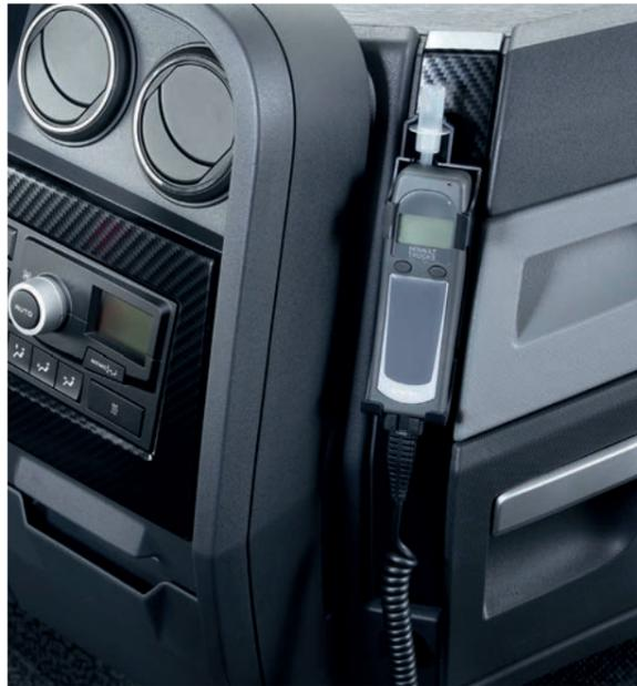
Breathalyser - Alcolock test, left-hand drive 74 23 253 861
