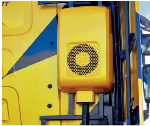
Cab interior temperature controller - SPX1200RT for **High Sleeper cab** 74 24 082 551
