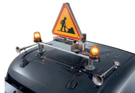
Worksite bar equipped with warning triangle and rotating beacons 74 21 650 717
